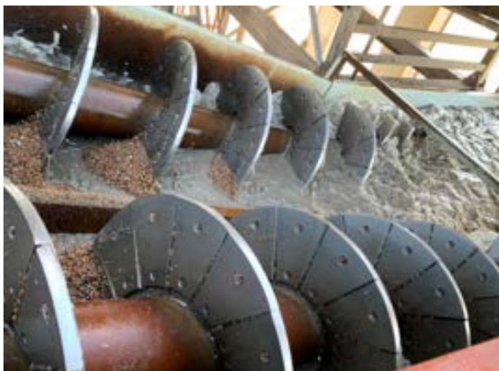
ABRASION-RESISTANT A-532 WEAR PADDLES & SHOES
